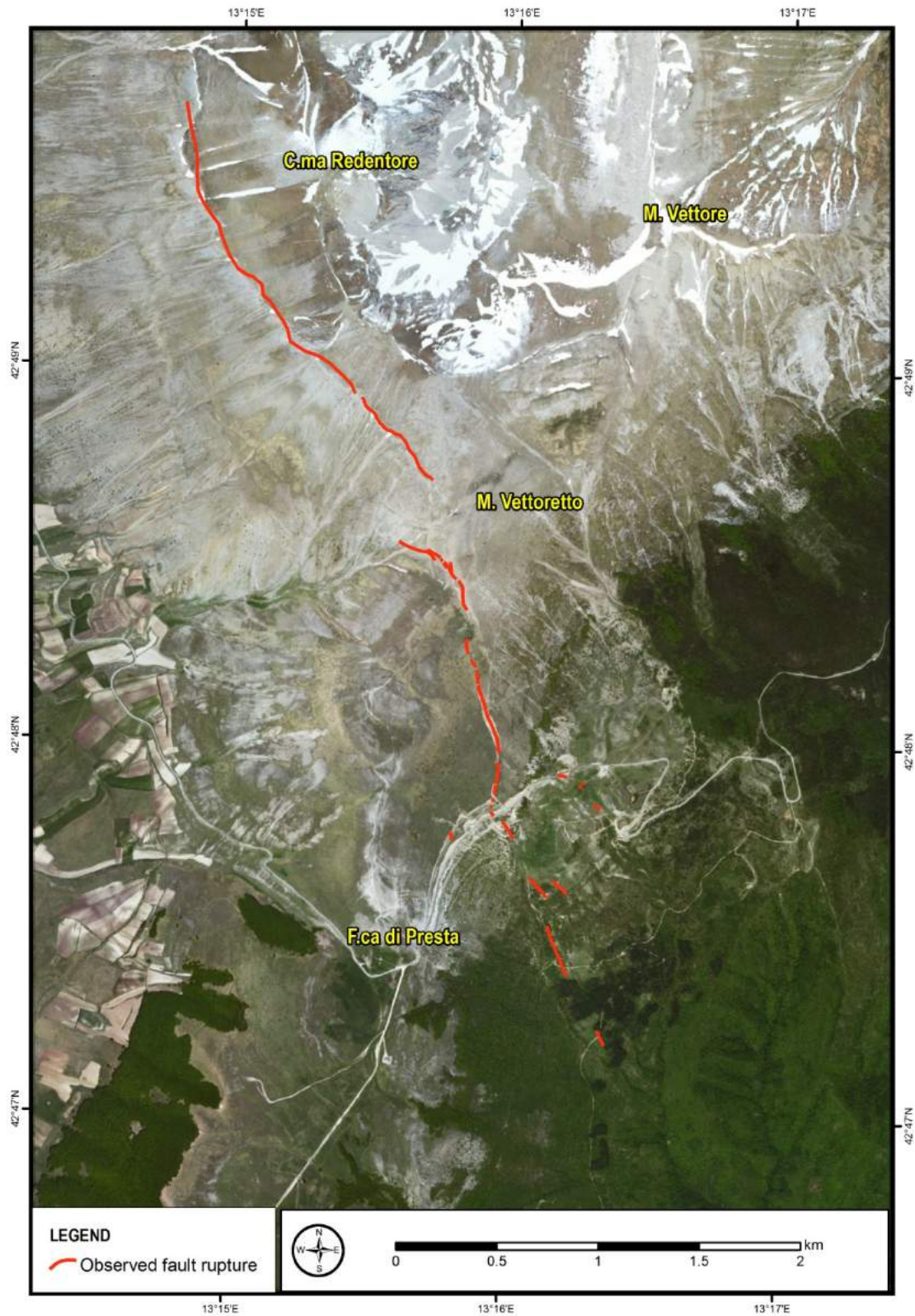
Fig. 15 – Pattern of ground ruptures observed along the Mt. Vettore fault. See text for details.
