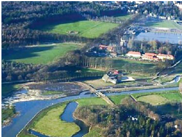
River Mark, Breda, the Netherlands: floodplain restoration project, just upstream of Breda, known as “Bieberg”, incorporates re- meandering and secondary bypass channels
